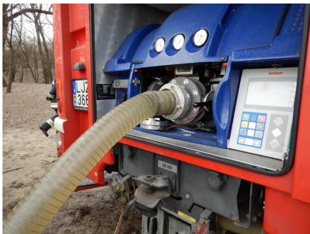
Picture 1 - Filling a fire engine from open water source, from the river Danube (Source: Péter Pántya)
